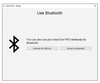
N.B. If you do not see the option to connect via Bluetooth at this point, your PC or operating system does not support Bluetooth LE (Low Energy). In this case, you must connect the Seal One device to your PC via USB.
